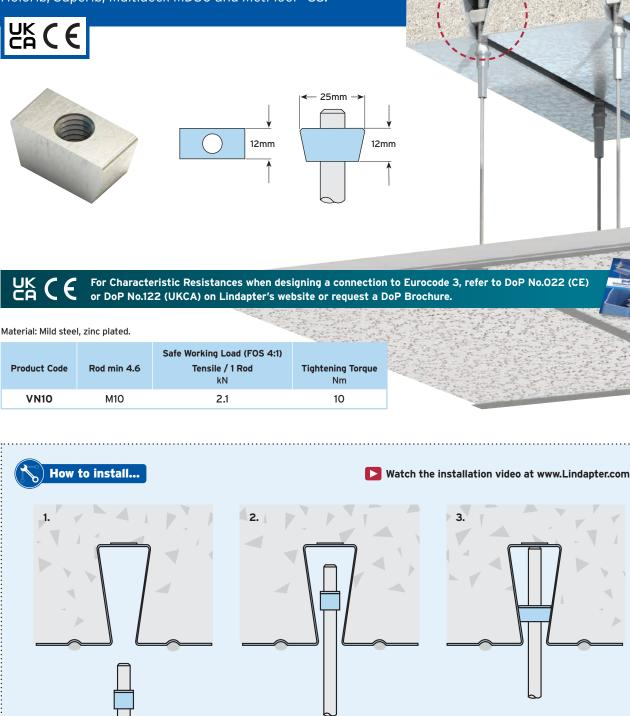
1) Screw the V-Nut (VN) onto the threaded rod.
