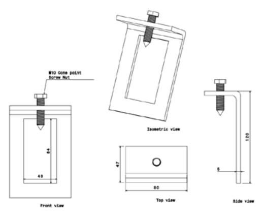
41x82mm Channel Beam Clamp
