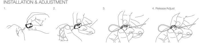
Ensure a minimum 75 mm of tail wire exits the hanger.
